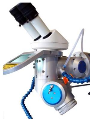
From the vertical working position the processing head with binocular can be pivoted sideways up to **120°** to the left and right allowing the laser beam to be deflected in nearly every position.
