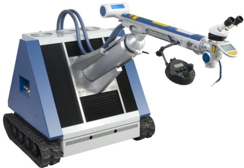
With the welding laser *ALFLAK mobile* deposit welding and welding of contours can be accomplished safely and efficiently on **big machine components, design parts** and **injection- and forming dies**. The new semi-automatic „**User-Coordinate-Controller**“ makes **three-dimensional** motions very easy.
