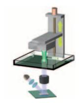
The DLP Projection method is characterised by high accuracy and a high productivity, the main features of the DigitalWax 009J.
