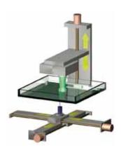
The Plotter X-Y scanning method is characterised by high accuracy and a relatively small productivity, the main features of the DigitalWax 008J.
