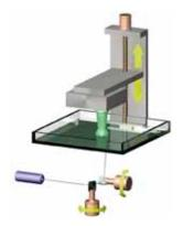
The Galvanometer type scanning method allows the highest building speed and accuracy and is adopted by DigitalWax 028J, 028J+, 029J, 029J+, and 030J systems.
